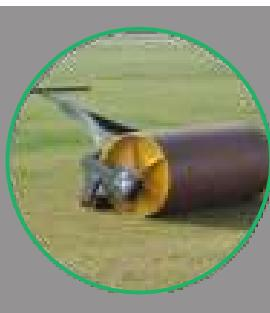
Manual Rollers (500 Kgs – 1 Ton)- Our Manual rollers are crafted from quality thick metal sheets, We provide an additional small roller attached with the main rolling wheel and also our rolling handle is fixed four feet above to make it easy to operate by a single individual.
